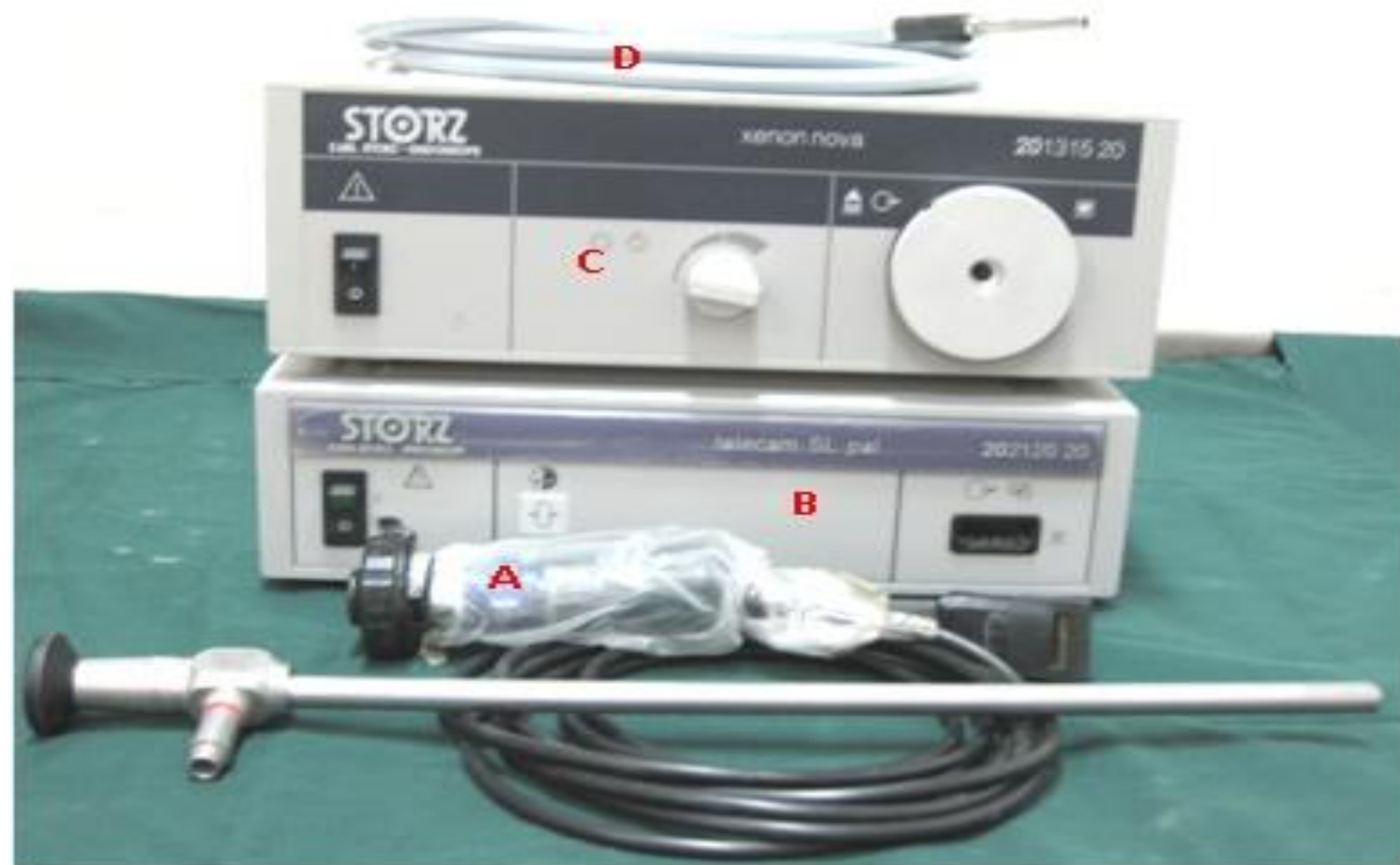
Fig.2: Laparoscopic video-camera system: head of camera(A),camera control unit(B),light source (C), light cable(D).
